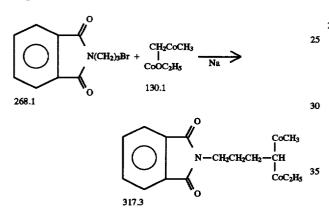
In a three-neck flask having a capacity of 500 ml, provided with  $CaCl_2$  cooling there are dissolved 4.60 g (0.2 g/A) Na in 100 ml anhydrous ethanol. To the solution, at room temperature, there are added 27.32 (0.21 moles) of [acetacetic esther] acetoacetic ester and then, after ten minutes, 40 g of 3-bromopropylphthalimide and, after one hour, further 12.5 g (in total 52.5 g corresponding to 0.196 moles), by holding the reflux processing and continuing for further three hours.
